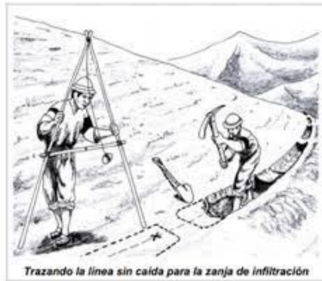
Figure 4. Water draining into ditches stays in place longer, allowing time for slow filtration into deeper layers of soil. Source: JALDA, 2009
